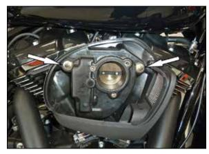
5. Remove the two breather/air filter base mounting bolts as shown.
