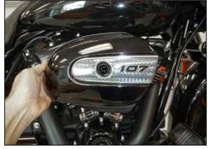
2. Remove air filter cover bolt and air filter cover as shown.
