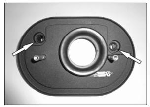
9. Install the remaining two o rings onto the front of the K&N® back plate as shown.
