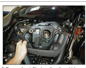
6. Remove the air filter base from the vehicle as shown
