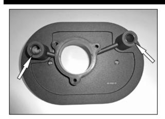
8. Install two of the o rings provided onto the back side of the K&N® back plate as shown.
