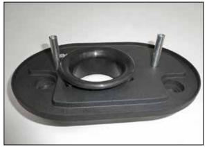
7. Install the provided intake velocity stack and the three throttle body bolts in the K&N® back plate. Install the two filter spacers onto the front of the K&N® back plate as shown using the provided hardware.
