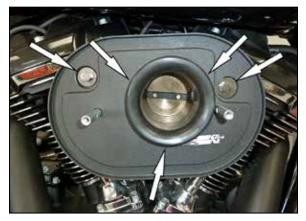
10. Install the filter back plate onto the throttle body and secure first with the throttle body bolts and then with the breather bolts.
